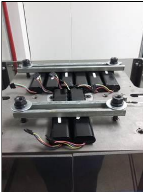
Photograph 7: Shock Test Setup –Fore/Aft, Negative Direction
