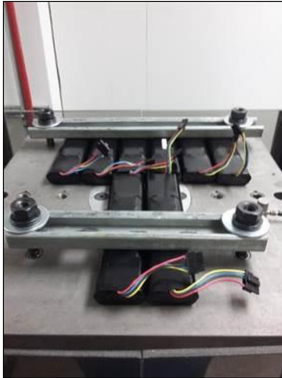
Photograph 6: Shock Test Setup –Fore/Aft, Positive Direction
