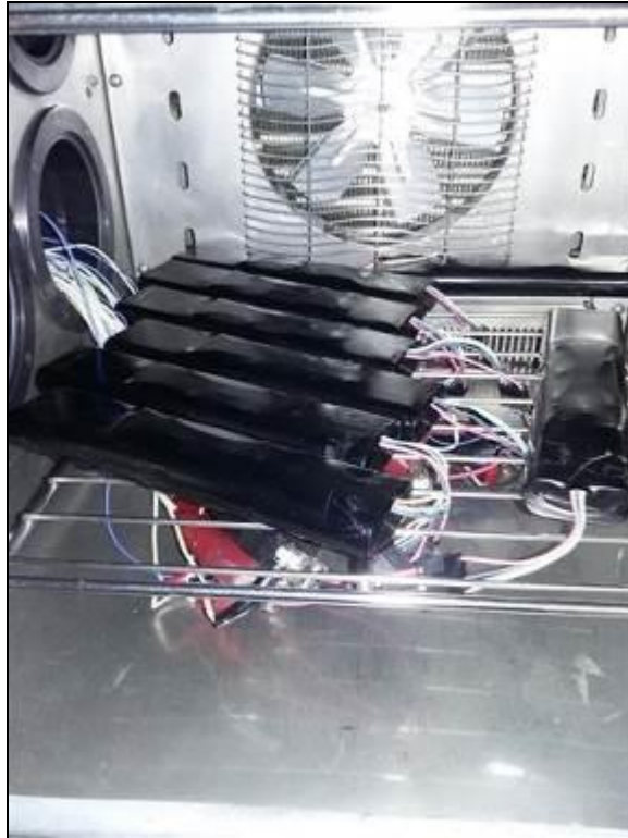
Photograph 14: Overcharge Test Setup
