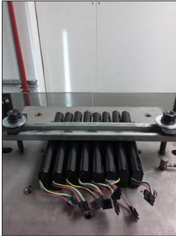
Photograph 8: Shock Test Setup – Lateral, Positive Direction
