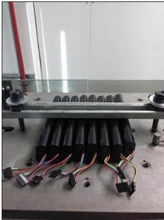
Photograph 9: Shock Test Setup – Lateral, Negative Direction
