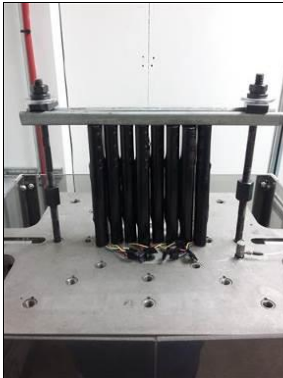
Photograph 11: Shock Test Setup – Vertical, Negative Direction
